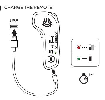
NOTE: If the remote is charged every time the board is charged it should take much less time to charge.
